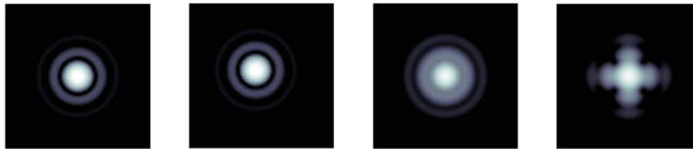
(b) Focal plane images for low order wavefront aberrations.
